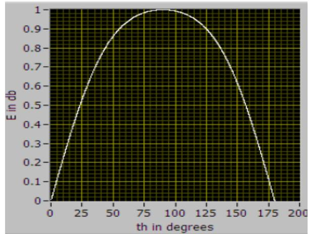
Fig. 10. Radiation pattern of microstripAntenna in H- plane at 10GHz in labview with  $\theta$  value on x-axis and electric field on y-axis
