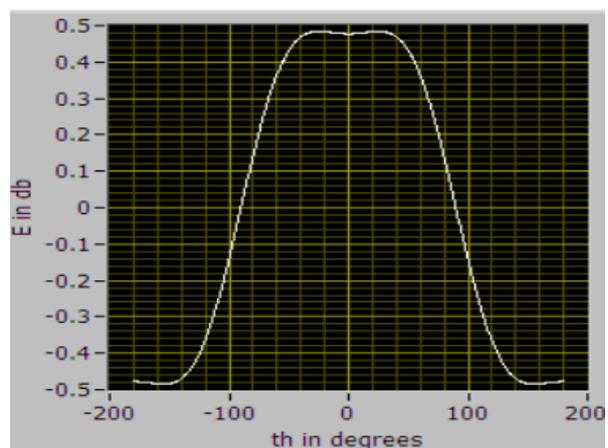
Fig. 7. Radiation pattern of microstripAntenna in E-plane at 10GHz in labview with  $\theta$  value on x-axis and electric field on y-axis
