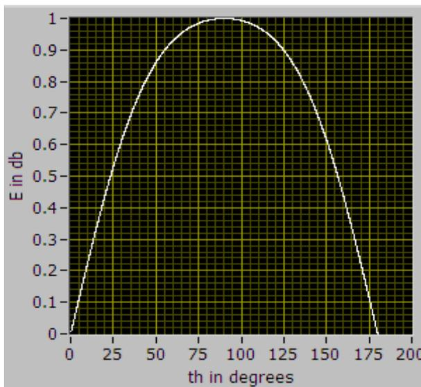
Fig. 9. Radiation pattern of microstripAntenna in H- plane at 10GHz in labview with  $\theta$  value on x-axis and electric field on y-axis
