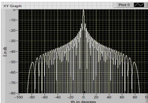
Fig. 14 Radiation pattern of microstrip array for 40 elements with  $\theta$  value on x-axis and electric field on y-axis
