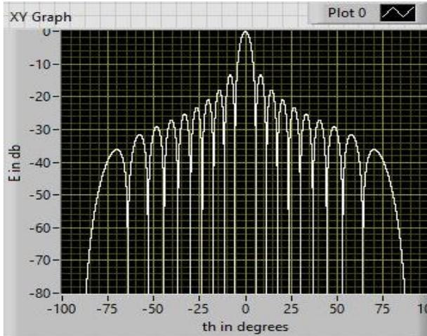
Fig. 13. Radiation pattern of microstrip array for 20 elements with  $\theta$  value on x-axis and electric field on y-axis
