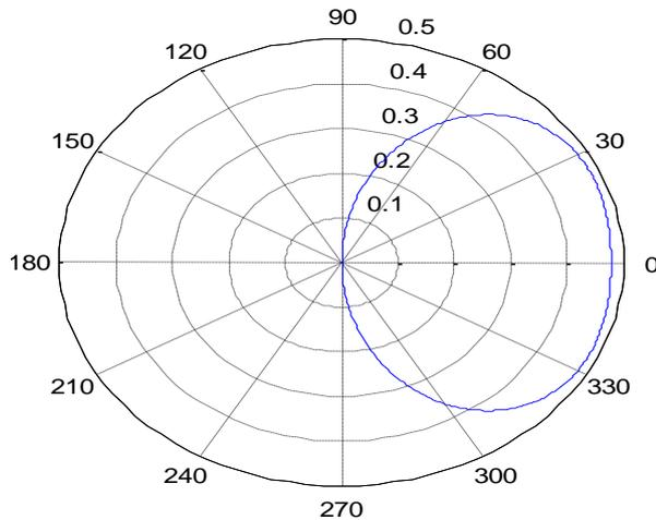
Fig. 3 Radiation pattern of Microstrip Antenna in E-plane at 10GHz
