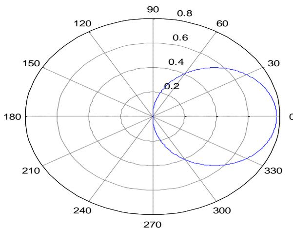
Fig. 4.Radiation pattern of microstripAntenna in E-plane at 30GHz
