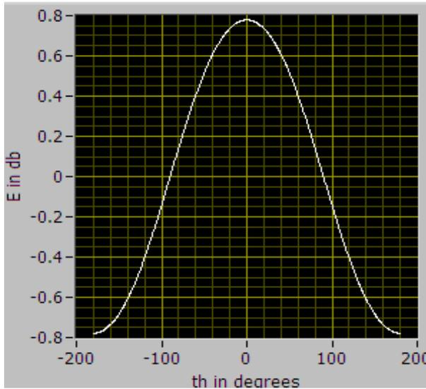
Fig. 8. Radiation pattern of microstripAntenna in E-plane at 30GHz in labview with  $\theta$  value on x-axis and electric field on y-axis
