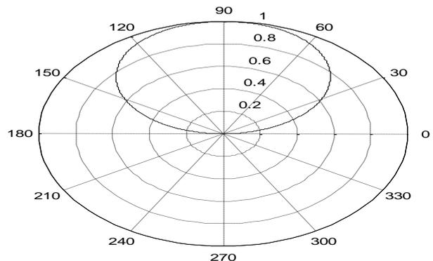
Fig 6 Radiation pattern of microstripAntenna in H-plane at 30GHz
