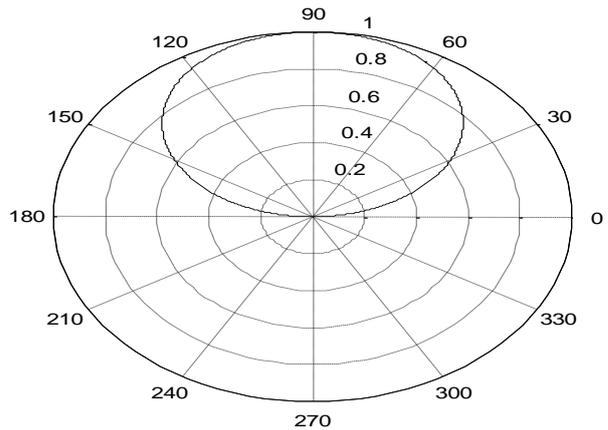
Fig. 5 Radiation pattern of microstripAntenna in H-plane at 10GHz
