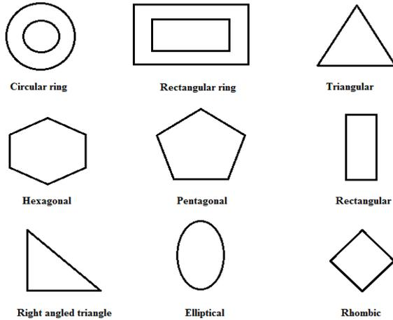
Fig 1 Different shapes of microstrip patch elements.
